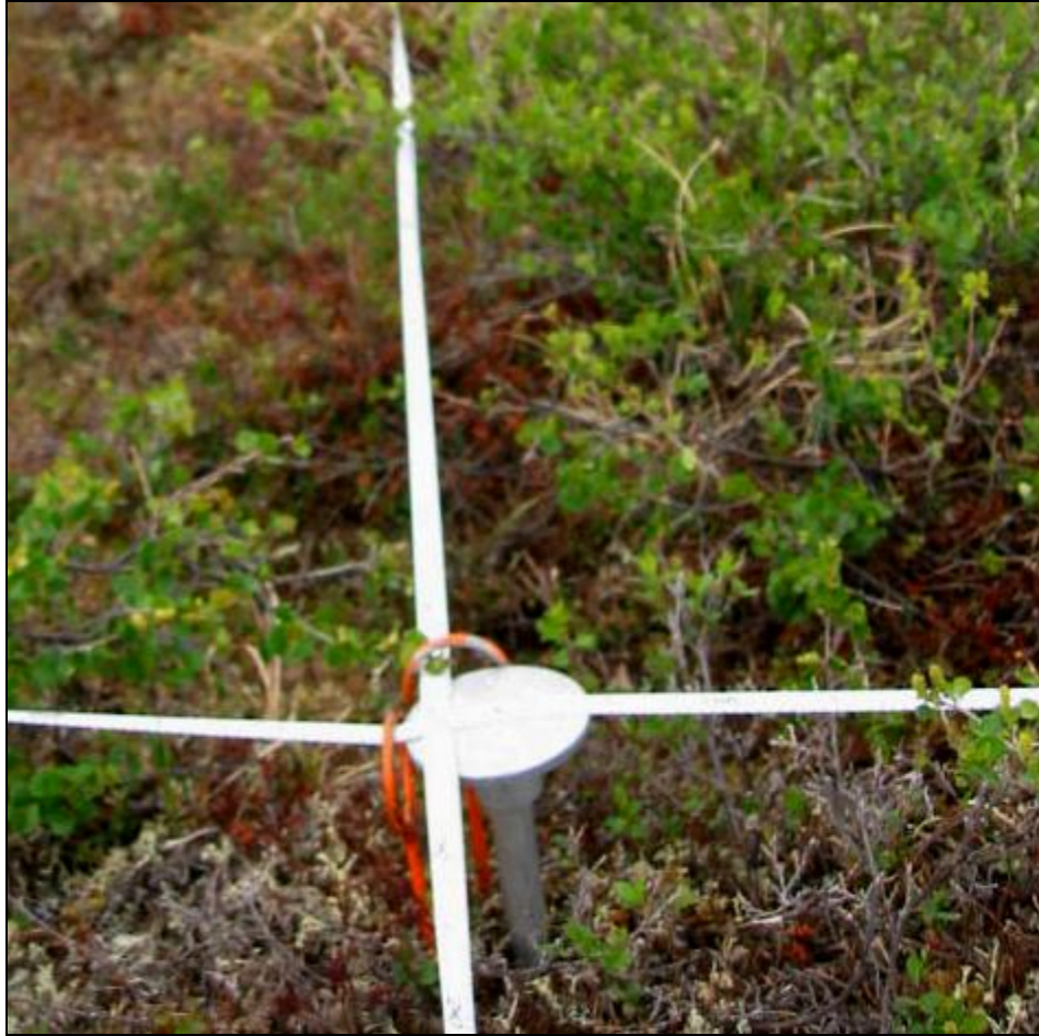
Figure 7. Plot monument used for marking permanent vegetation monitoring plot centers.
