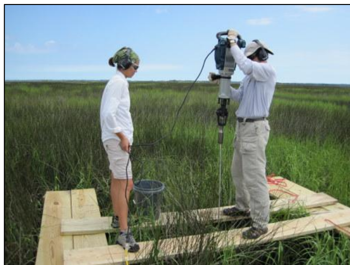
Figure 9. NPS staff installing a RSET monitoring station.
