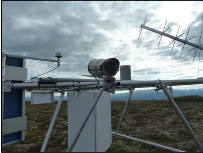
Figure 10. Coville RAWS – Campbell Scientific time-lapse camera set-up.
