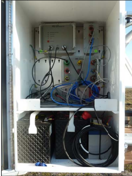
Figure 5. Contact Creek RAWS - The inside of the instrument enclosure photographed just before departure. Additional 35 Ah battery for Campbell Scientific time-lapse camera is visible in the lower-right portion of the photograph.
