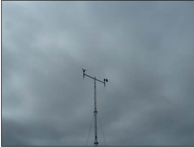
Figure 8. Coville RAWS – Wind direction sensor with no tail.
