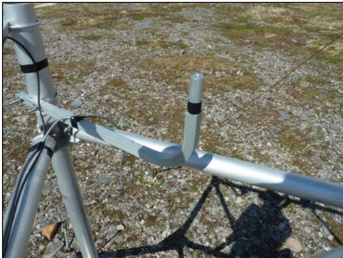
Figure 12. Fourpeaked RAWS – AT-RH sensor was missing.
