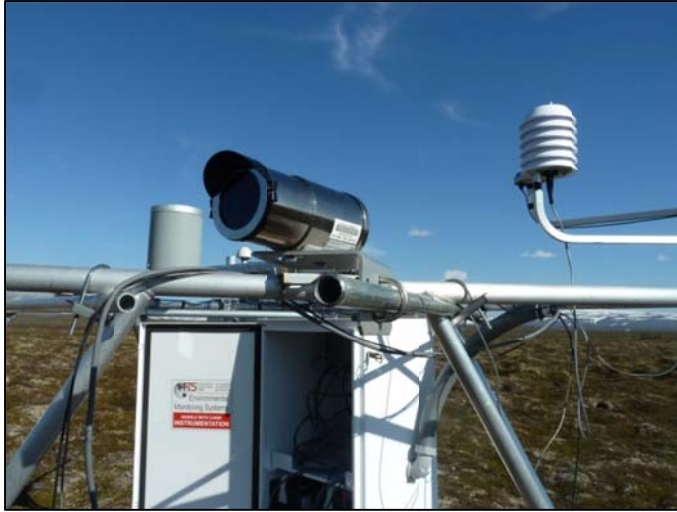
Figure 7. Contact Creek RAWS – Campbell Scientific time-lapse camera set-up.
