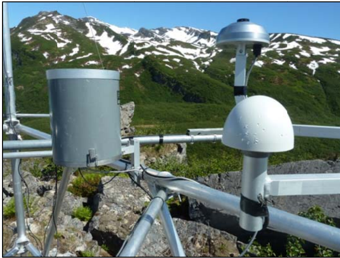
Figure 22. Hickerson Lake RAWS – GPS antenna with bear teeth marks.
