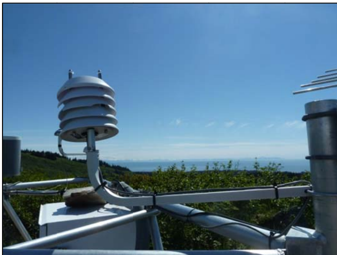
Figure 23. Hickerson Lake RAWS – Damage to the plastic louvers on the AT-RH sensor.
