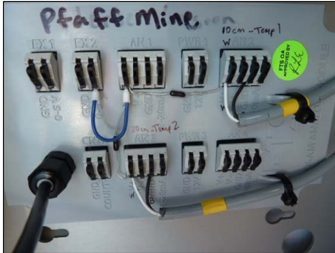
Figure 40. Pfaff Mine RAWS – Wiring configuration used on the analog/digital convertor to accommodate the dual soil temperature sensors.
