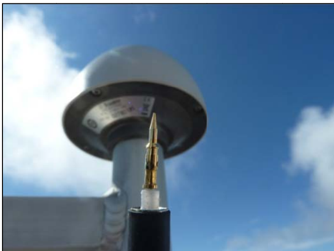
Figure 12. Fourpeaked RAWS – AT-RH sensor was missing.
