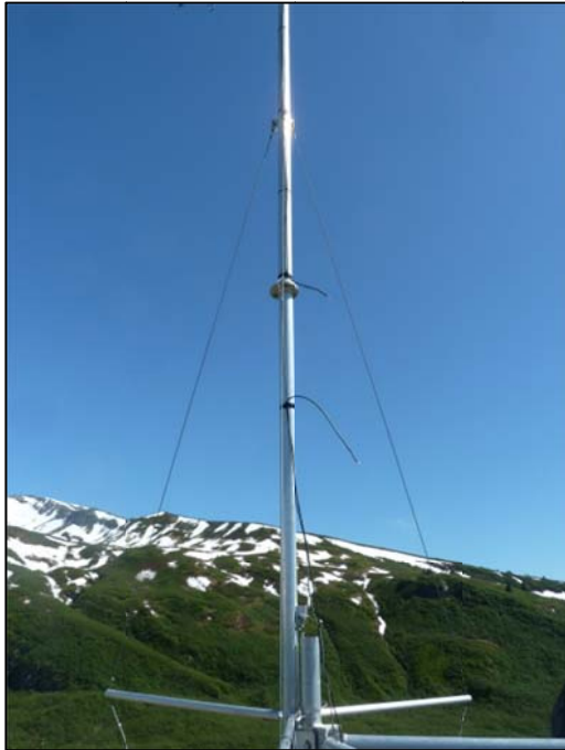
Figure 24. Hickerson Lake RAWS – The wind speed cable was cut, likely because it was pulled.
