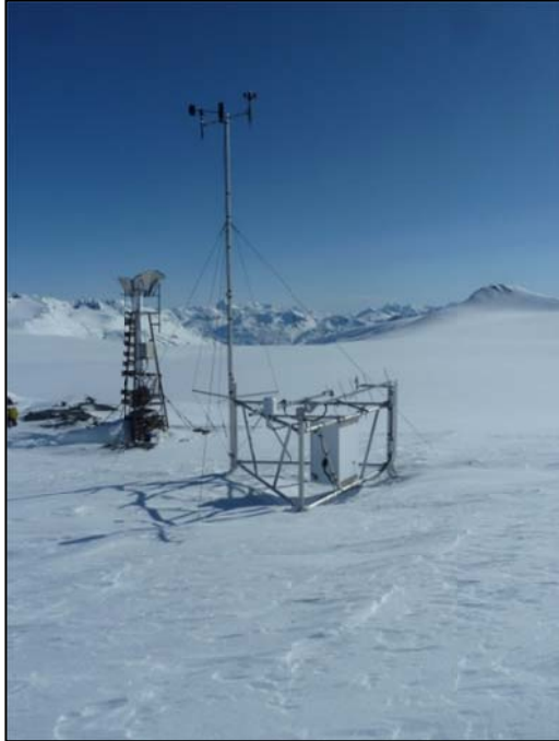
Figure 18. Harding Icefield RAWS – The weather station upon arrival with two feet of snow on the ground. The station is, in fact, level. The snow surface is sloping.
