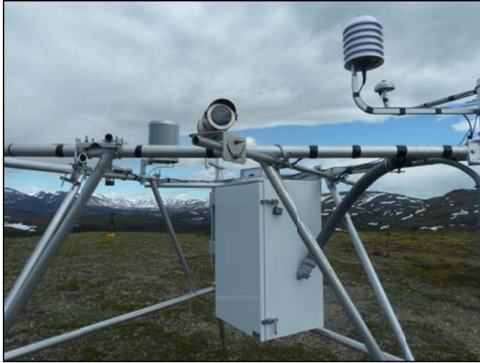
Figure 44. Snipe Lake RAWS – Campbell Scientific time-lapse camera set-up.
