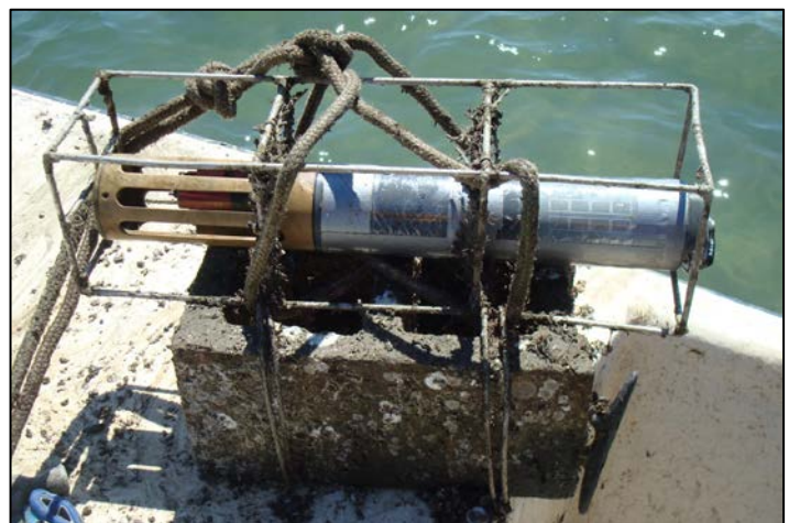
Figure 2. Photo of continuous data collection station in Middle Marshes (CALO 02) at Cape Lookout. Photo by John Fear, NC National Estuarine Research Reserve.
