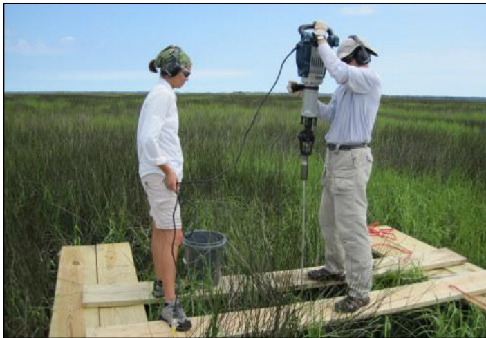
Figure 9. NPS staff installing a salt marsh elevation monitoring station.
