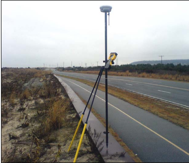
Figure S1.1. The Trimble R8 GNSS receiver and Trimble TSC2 field survey controller (Sandy Hook, November 2009).
