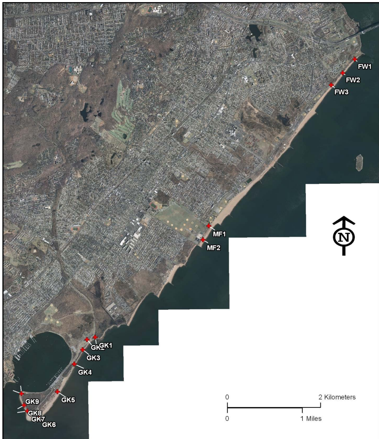
Figure 20. Spatial network of survey monuments and profile lines at Great kills (GK), Miller Field (MF) and Fort Wadsworth (FW), Staten Island Unit of Gateway National Recreation Area, NY.
