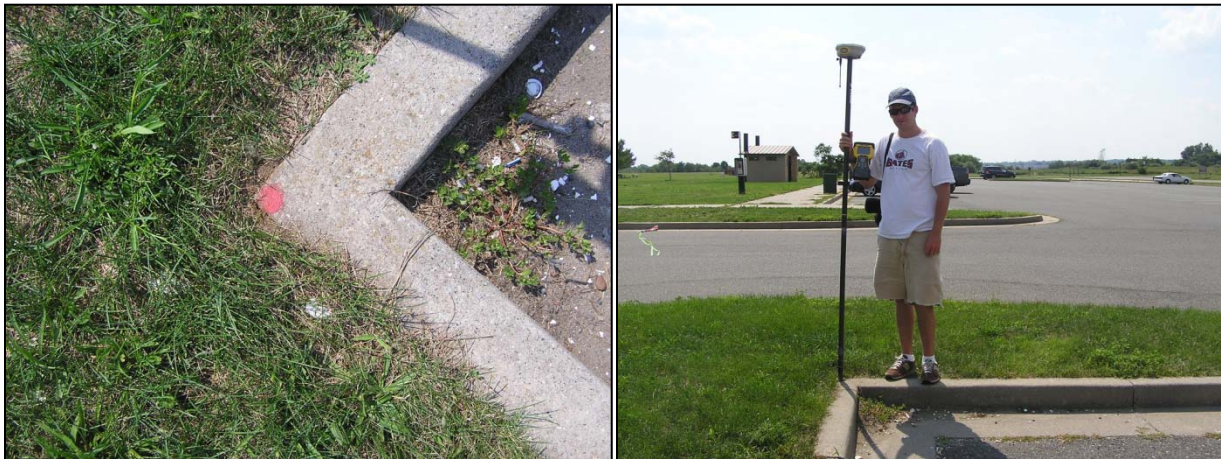
Figure S2.4. Benchmark location at corner of curb of a traffic island on a parking lot at Great Kills, GATE; adequate space for a GPS base station or rover receiver pole (Staten Island, August 2008).
