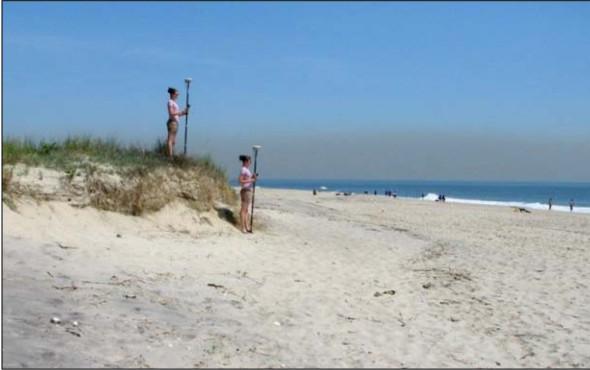
Figure S5.6. Measurement of topographic points along the profile line. Example of points being measured at change in slope: at top and bottom of the feature (Sandy Hook, May 2010).
