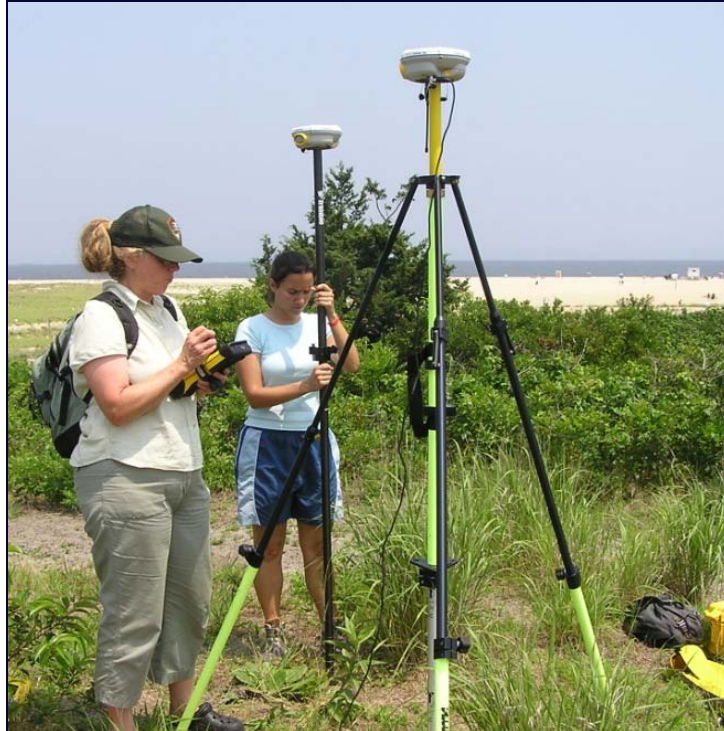
Figure 13. Trimble R8 GPS unit (base receiver on tripod, and rover receiver on pole) used for conducting topographical surveys at Gateway National Recreation Area (Sandy Hook, July 2006).
