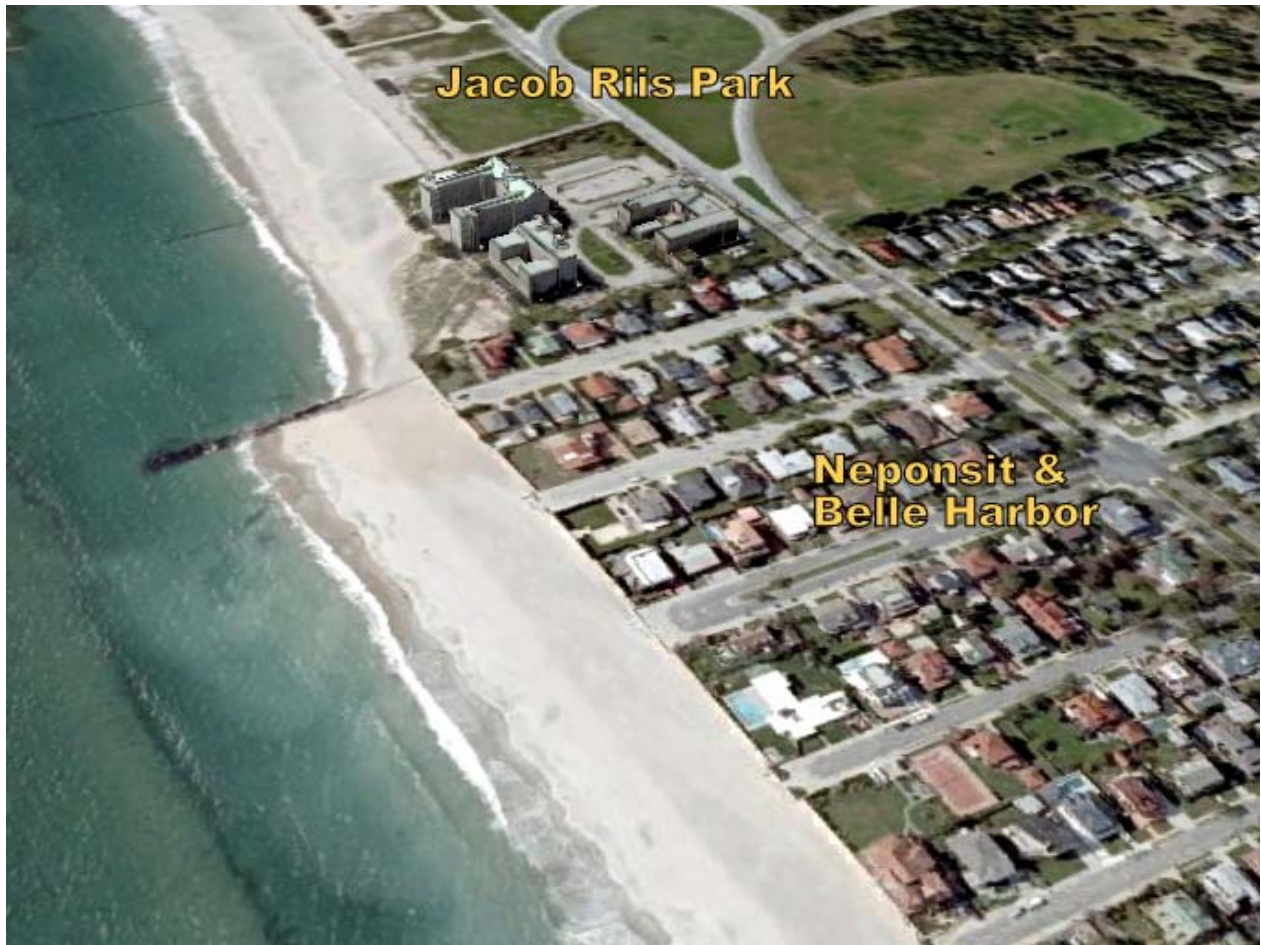
Figure 7. Groin between the Neponsit & Belle Harbor communities and Jacob Riis Park (GATE), causing sediment accumulation on the updrift side and erosion and inland beach displacement on the downdrift side. Aerial image accessed February 2010 at bing.com/maps/
