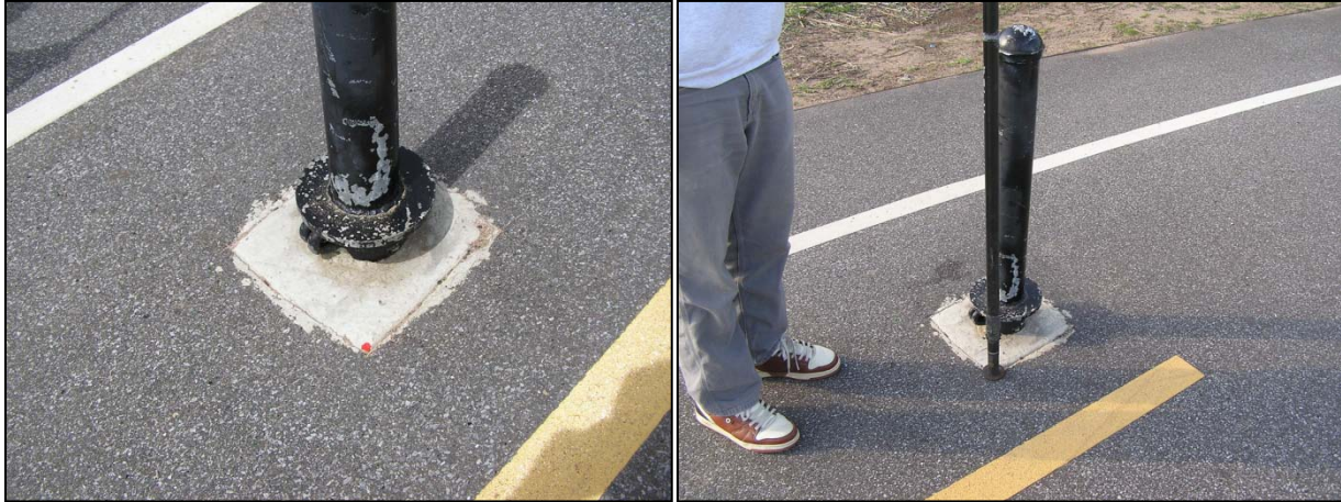
Figure S2.3. Benchmark located at corner of cement slab on the bike path at Fort Wadsworth, GATE; adequate space to site a GPS rover receiver pole (Staten Island, April 2009).
