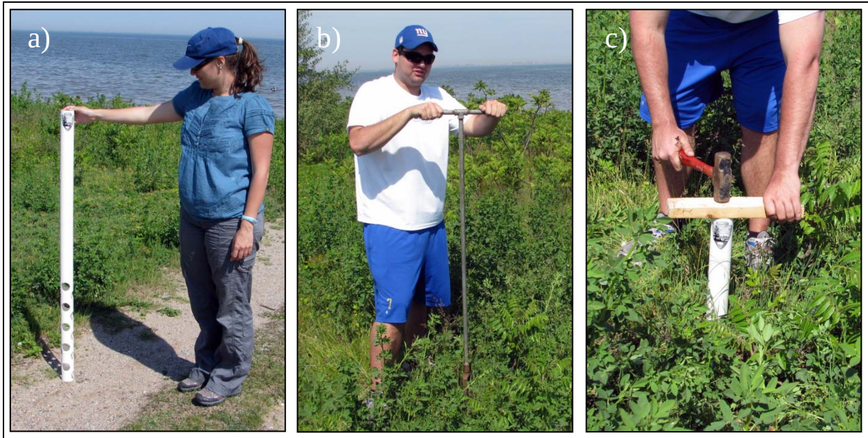
Figure S2.5. PVC pipe benchmark; a) PVC pipe with holes; b) Coring in field, and c) final driving of PVC pipe into sand.
