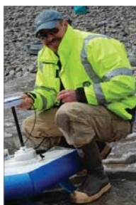
CAKN aquatic ecologist Trey Simmons readying an acoustic Doppler current profiler in the Nabesna River.
