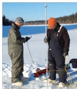
USFWS scientists measure flow in the Nabesna River through the ice, March 2012.
