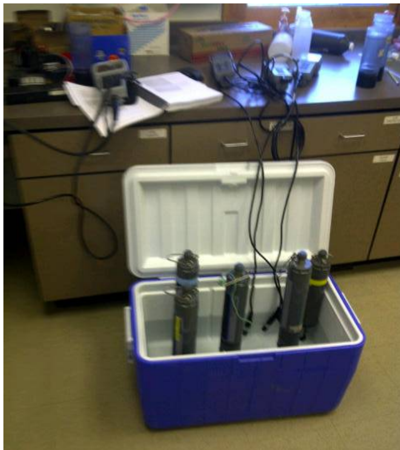
Figure SOP 3.2. Laboratory set up for temperature sensor comparison.
