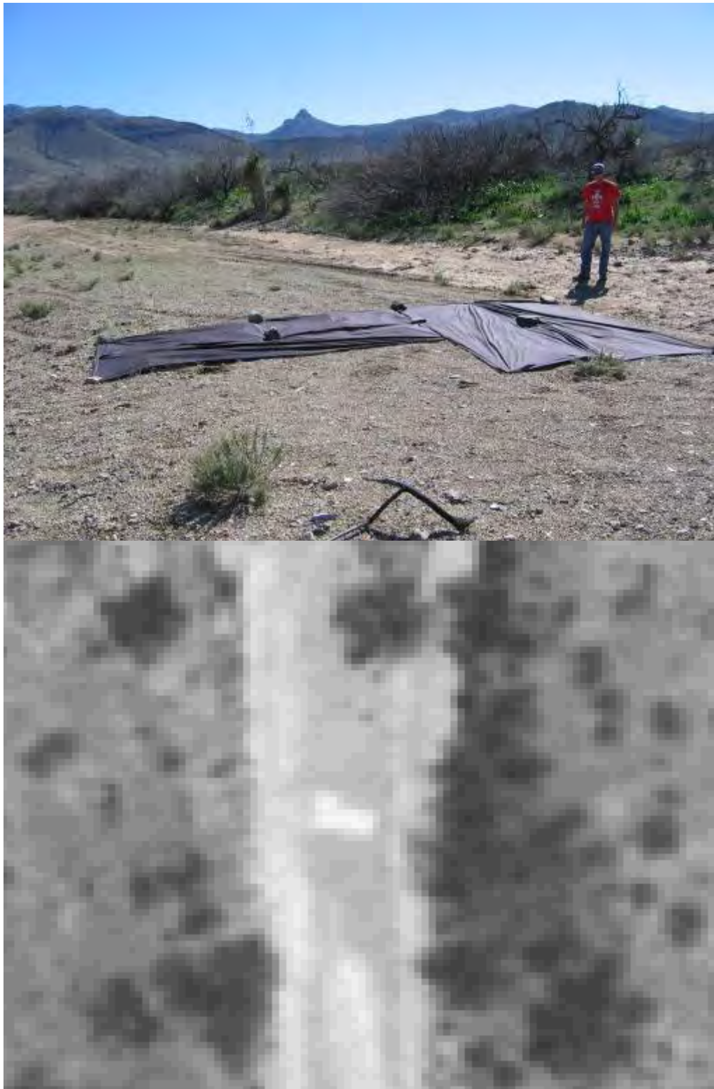
Figure 8. Black GCP target on the ground and in the Quickbird imagery.
