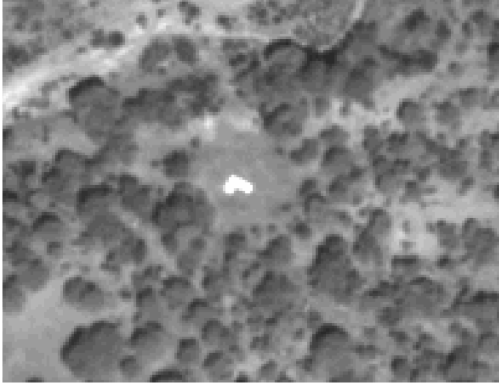
Figure 6. Satellite view of a white GCP target as recorded by Quickbird.
