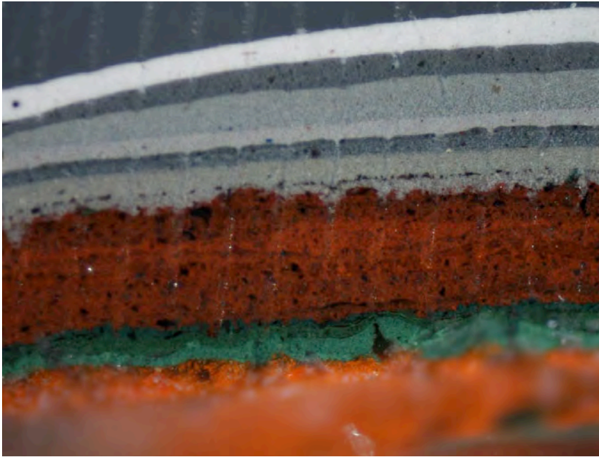
Figure 17. Cape Lookout Lighthouse. Photomicrograph of Sample CALO. I.3, removed from the astragal of the center cast iron column (at the Watch Level). Note the early red-orange primer followed by a dark green paint finish at bottom of photograph. This campaign may be original. Photograph by author, 100x magnification.
