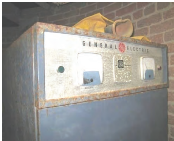
Figure C-63 Abandoned GE transmitter/receiver.
