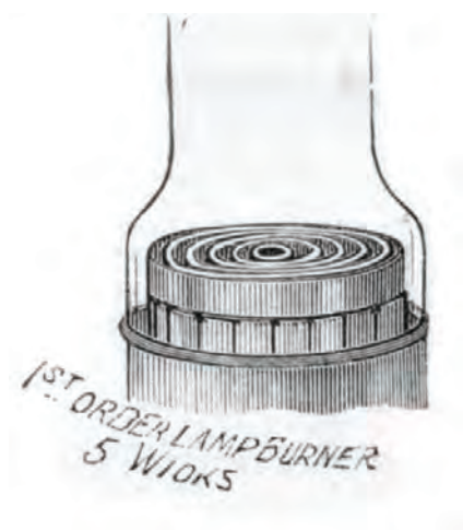
Figure A-5 Example of Argand reflector lamp (top) and 1 st Order Fresnel wick (bottom).
