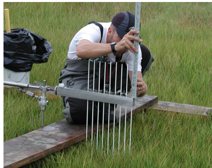
A SET is used to measure the surface elevation of a marsh. NPS photo.
