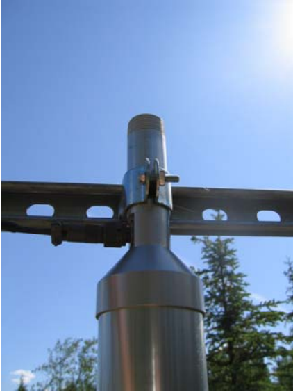
Figure 2. Close up shots of mounting devices on CAKN stations
