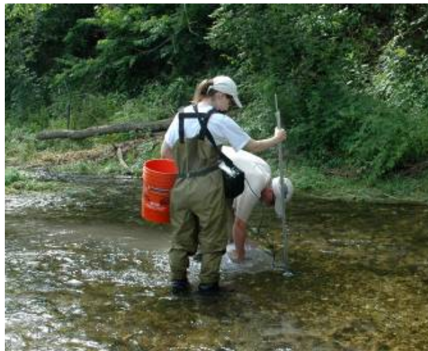
Figure 2. Measuring depth and current velocity in front of a sampling frame.
