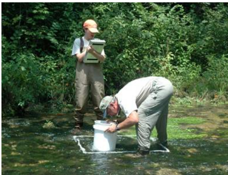
Figure 1. Placement of the sampling frame on the stream bottom and using a view bucket to assess coverage. A second team member records data.
