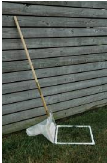
Figure 1. Invertebrate sampling net with sampling frame attached.
