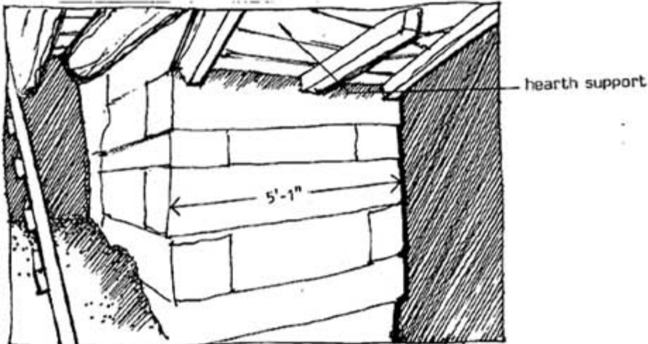
7A. Room 001 Cribbed timber chimney footing
