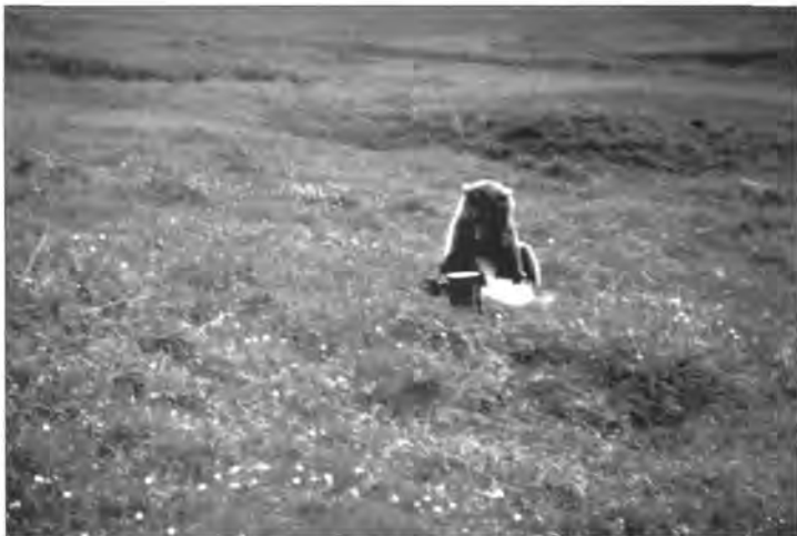
Field experiments with grizzly bears were conducted to test the effectiveness of different types of bear resistant food containers. NPS Interp. Collection, #5445, Denali National Park and Preserve
