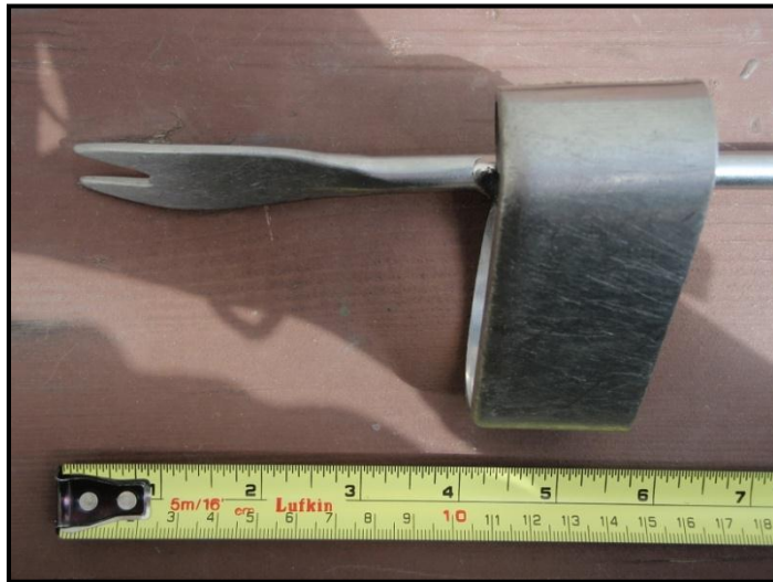
Figure 2. Compliance tool used near cultural resource sites to minimize possible damage to artifacts buried during control work.
