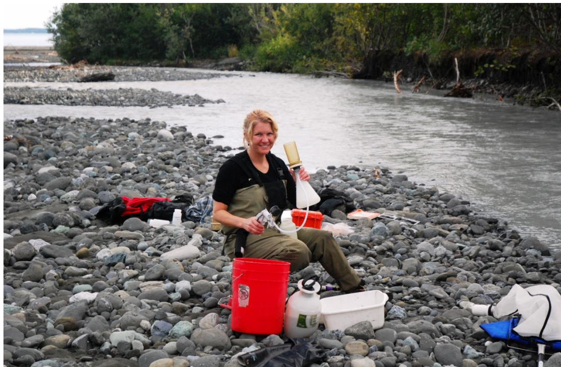
Figure 3. Filtering water chemistry samples in the field (Independence Creek, WRST).
