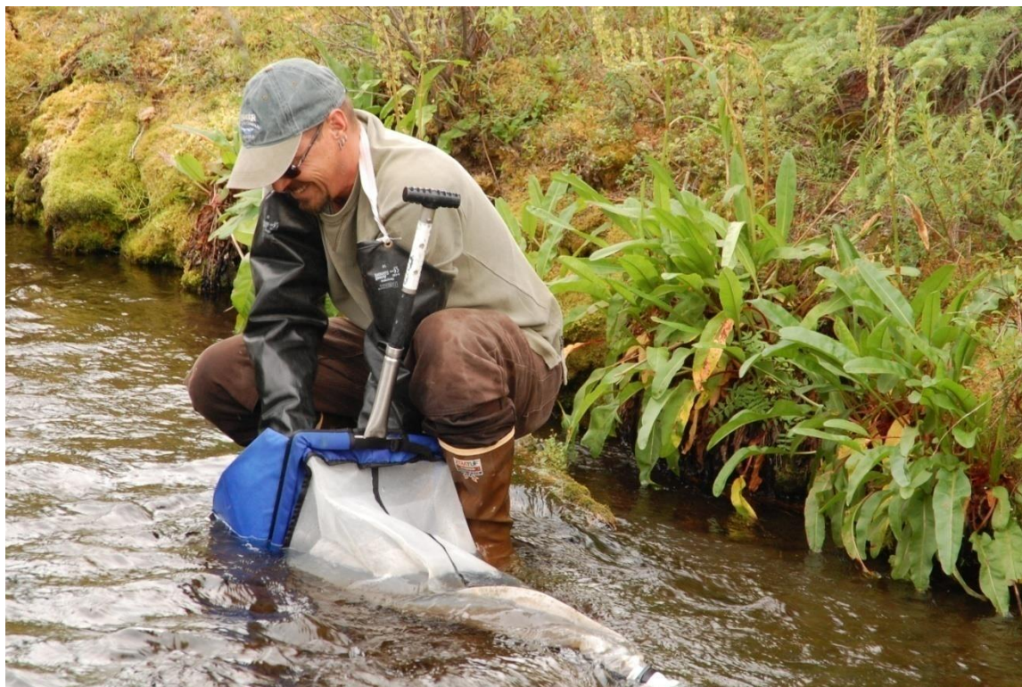
Figure 2. Collecting macroinvertebrates using a modified D-net (Rufus Creek, WRST).
