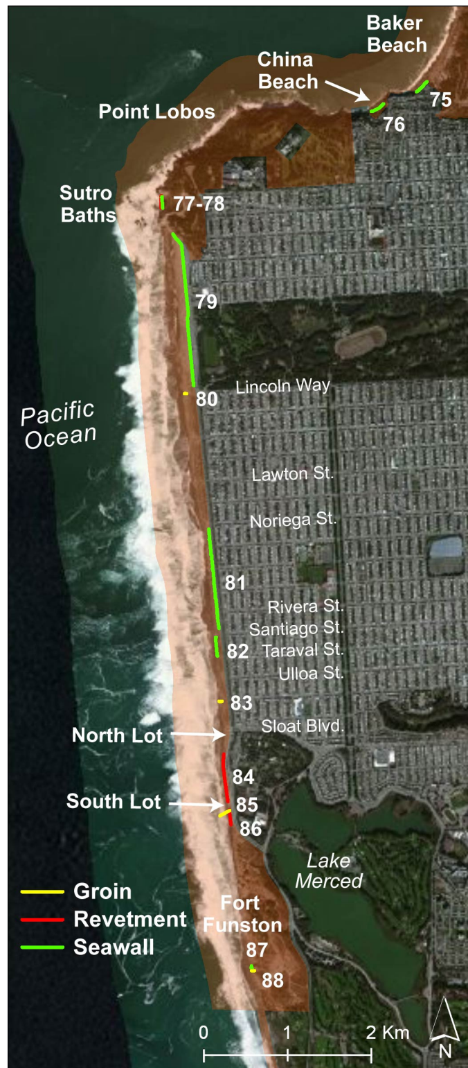
Figure 24. Baker, China, and Ocean Beach structure map. Orange shading shows park property. Groin #85, the Southwest Ocean Outfall pipe, extends 7.2 km (4.5 mi) offshore (not shown) and Groin #88, the Vista Grande Outfall, extends 762 m (2,500 ft) offshore (not shown) (image from ESRI Bing Maps basemap layer 2012).
