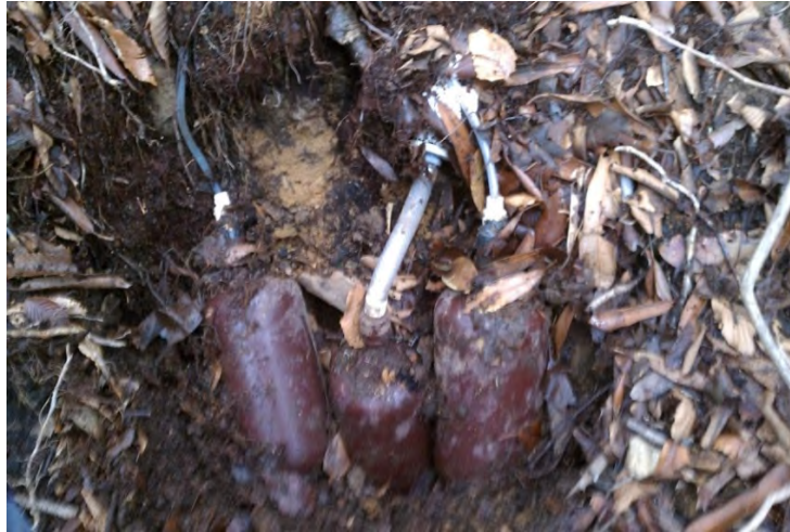
Figure 5-1. Photo of the soil lysimeter collector bottles at Rock Creek (Cosby) site.
