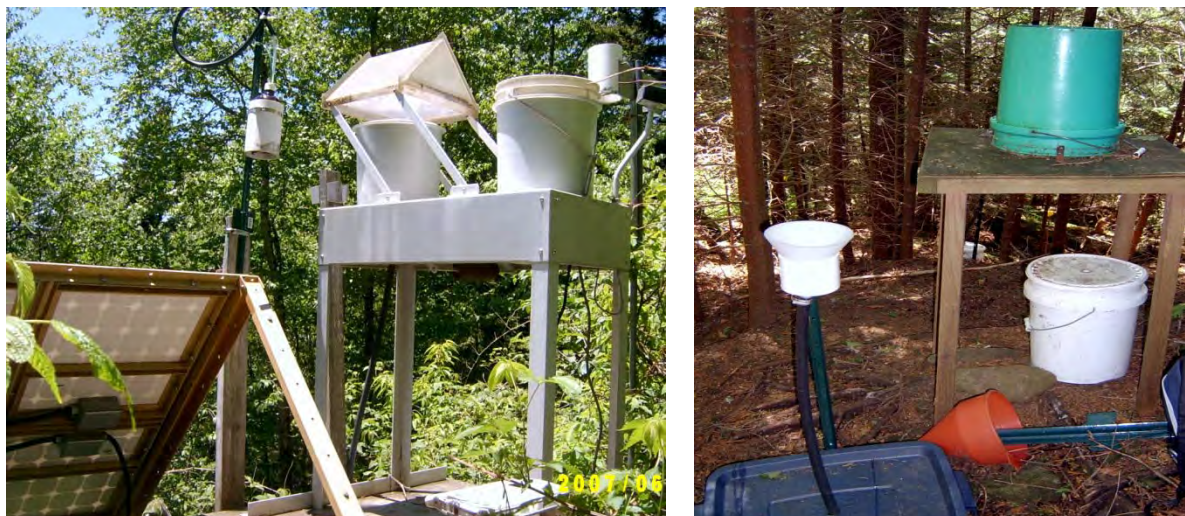
Figure 1-3. Photos depicting wet deposition collection (right) and throughfall collection (left).
