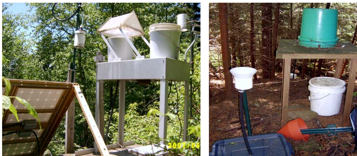
Figure 1-3. Photos depicting wet deposition collection (right) and throughfall collection (left).
