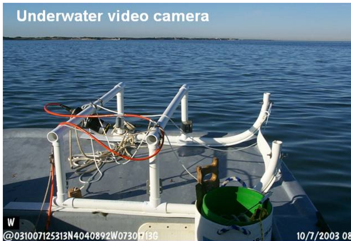
Figure 10. Underwater video camera attached to a sled and towed behind a vessel.
