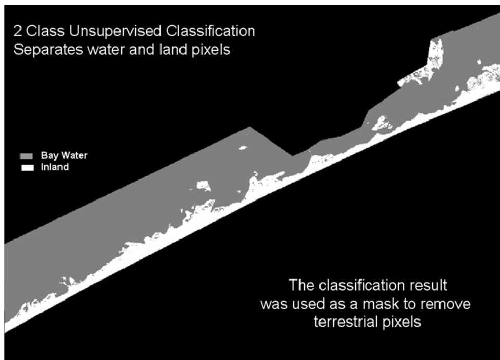
Figure 20. A section of the land-mask AOI created by a two-class unsupervised classification using only the near infrared band of the QuickBird-2 imagery data.
