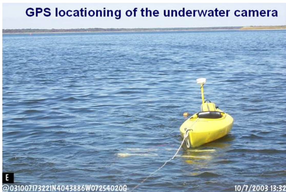
Figure 11. Trimble ProXR GPS receiver mounted on a kayak positioned directly over the camera sled.
