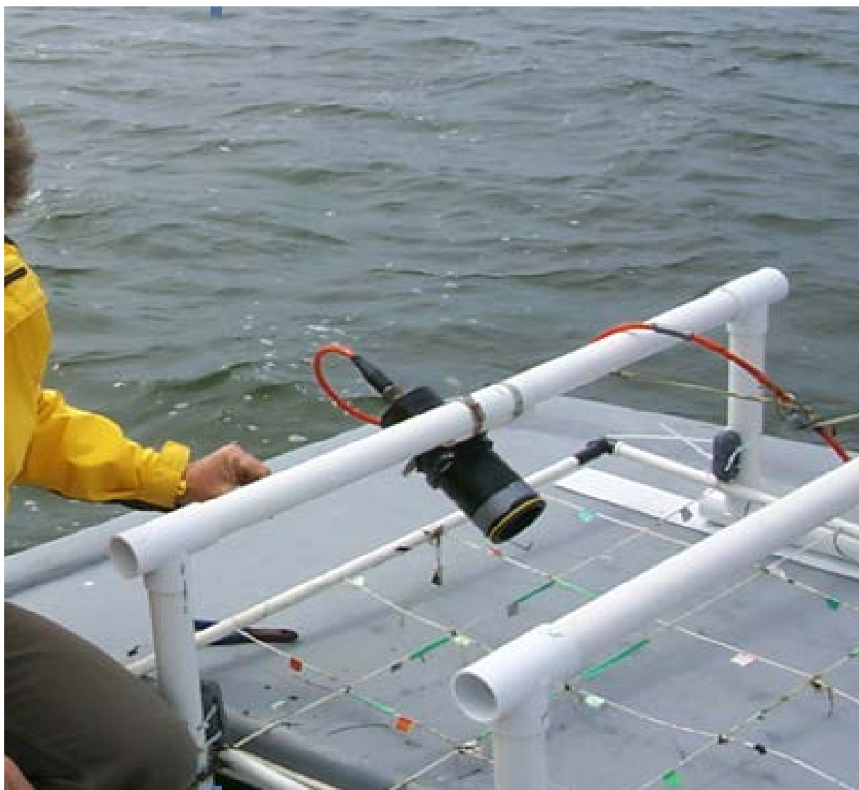
Figure 14. Gridded, 0.25m PVC frame used to estimate percentage cover of SAV.
