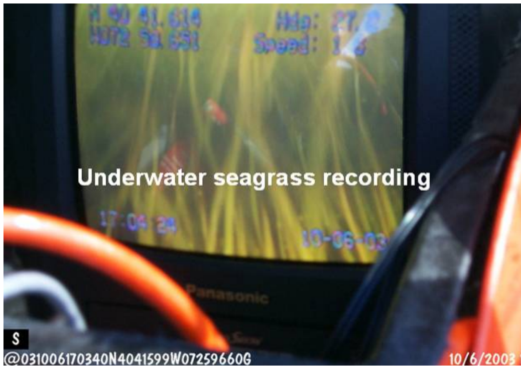
Figure 12. VCR/TV combo aboard the towing vessel recording SAV conditions and geographic coordinates on video files.
