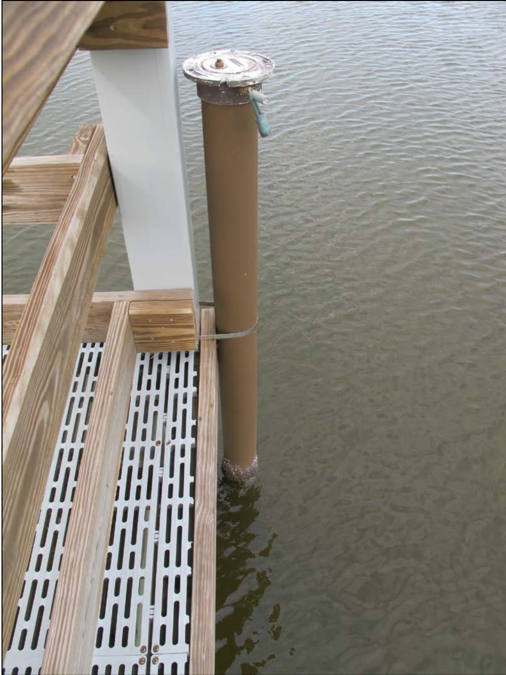
Figure 2. Continuous data collection platform at Canaveral National Seashore visitor center dock showing sonde housing and locking cap. Photo by Aaron Rinehart, SECN staff.
