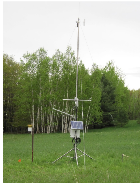
A remote automated weather station (RAWS) in Pictured Rocks National Lakeshore (Michigan).
