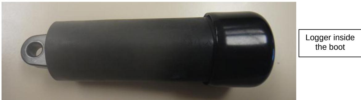
Figure SOP 3-1. HOBO® Water Temp Pro v2 logger inside boot and cap.
