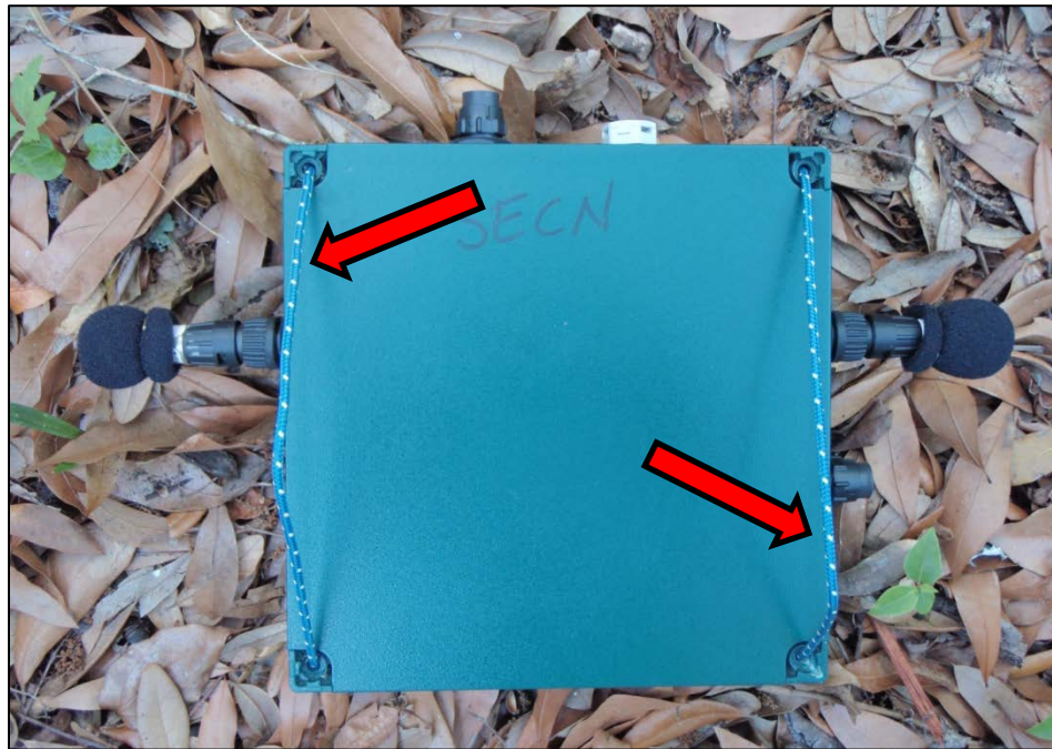
Figure 1. Utility-cord (3 mm) harness (red arrows) attached to the back of the automated recording device. Harness is affixed through the existing screw-hole mounts with an inside stopknot.
