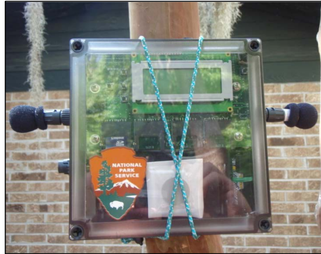
Figure 2. The mounting cords are fed through the harness on the automated recording device, wrapped around the mounting object, any extra cord is further wrapped around the device to ensure stability, and the utility cord is tightened with cordlocks (red arrows).
