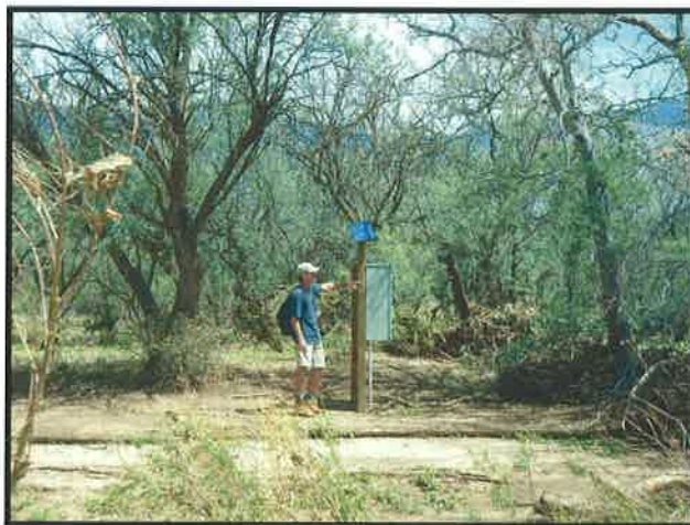
Figure 4. Data logger was nearly submerged. Water was 14.4 ft above channel bottom at this point.
