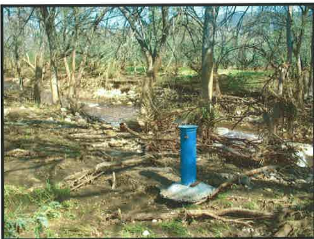
RC-4 was also topped (note high water mark on vegetation).
