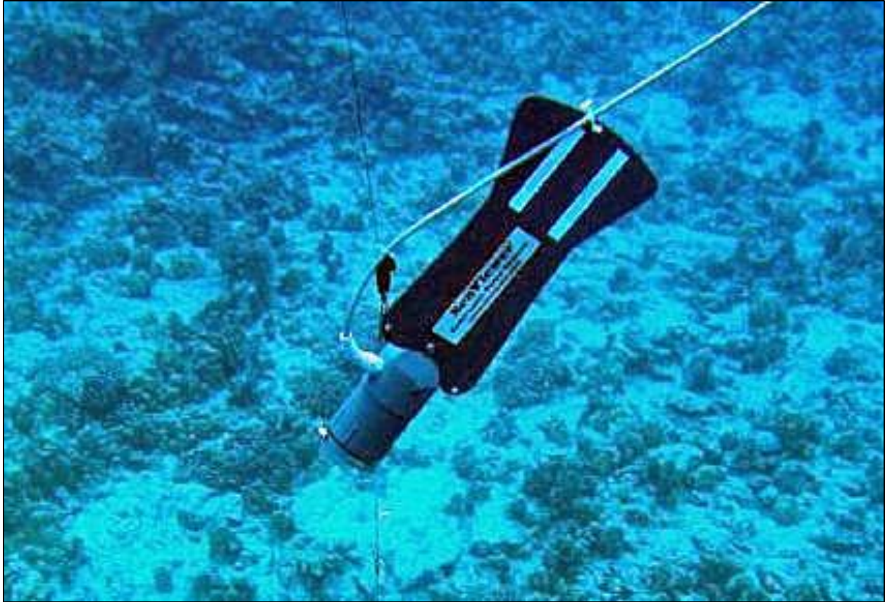
Figure 4. The Seaviewer Sea-Drop 950 drop-camera (pictured) was used by NOAA in benthic mapping projects in St John, U.S. Virgin Islands (from Zitello et al., 2009).
