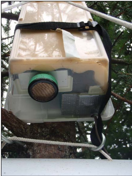
Figure 9. Complete bat detector installation with detector, housing, reflector, and battery.
