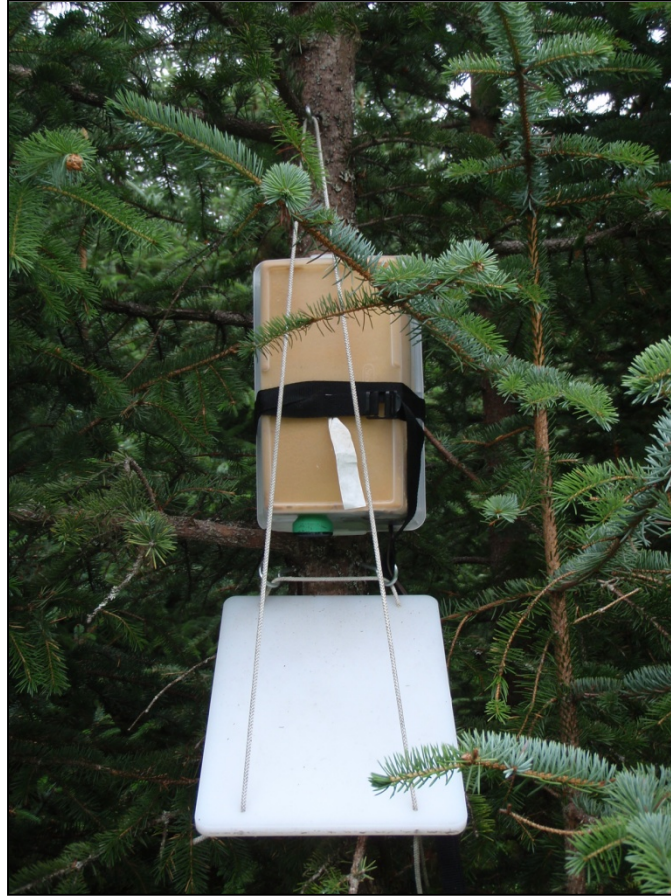
Figure 3. Bat detector with housing and reflector.
