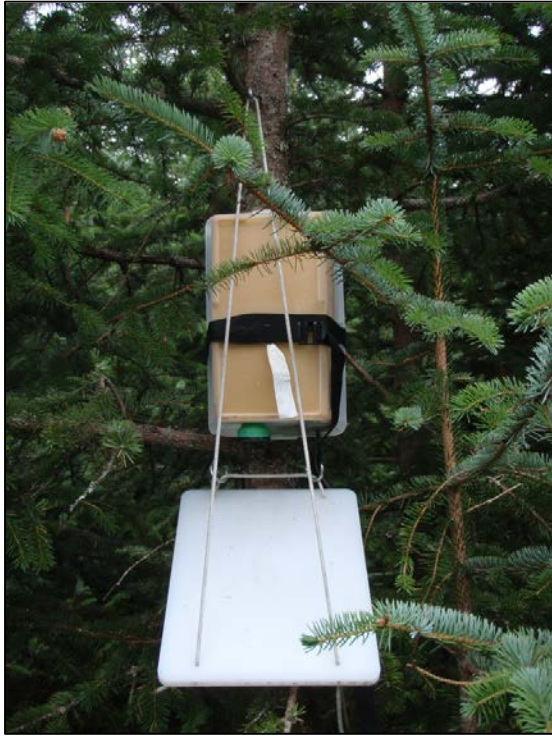
Figure 8. Bat detector installation with detector housing and reflector.
