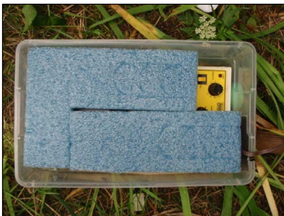
Figure 11. Detector with padding inside of housing.
