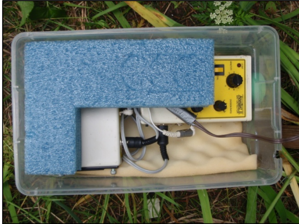
Figure 42. Detector with padding inside of housing.
