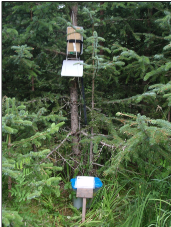
Figure 10. Detector in housing with microphone extruding from housing.
