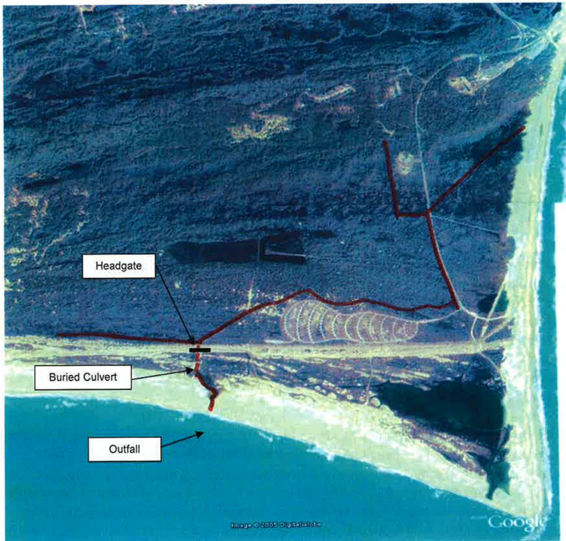
Figure 1. Major drainage ditches in the vicinity of the Cape Point Campground. When the headgate is open, water is drained from a large area of freshwater wetlands north and west of the campground. Additionally, when a ditch is opened to allow discharge to the ocean, water is drained from marine wetlands in the interdunal area south of the campground.
