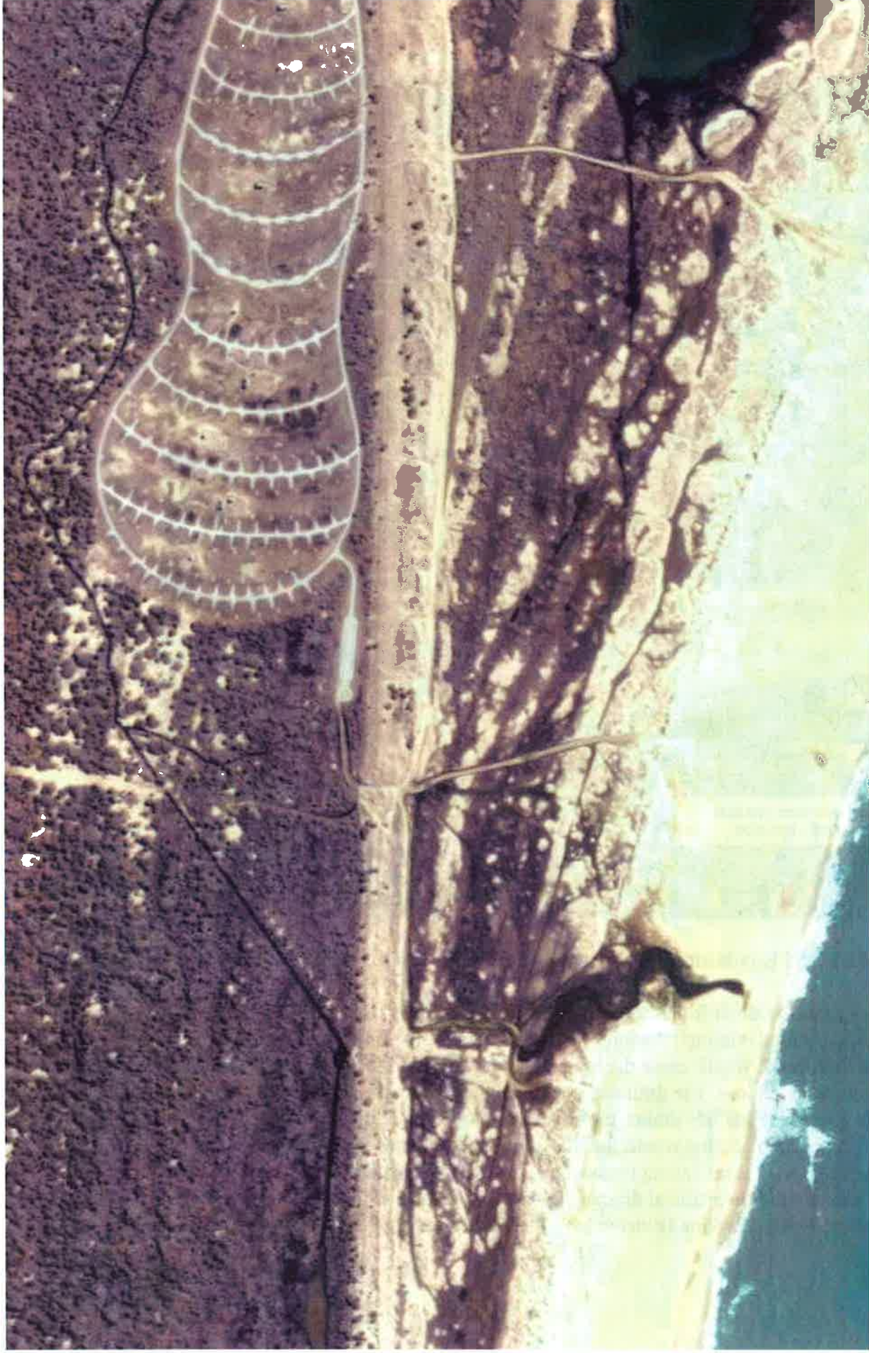
Figure 4. Detailed view of the area where interdunal roads are most susceptible to flooding. The main drainage ditch can be seen north of the primary dune and north of the campground. On this photo the outfall pond nearly reaches the ocean. In November 2005, the most seaward extent of the outfall pond is about coincident with the vegetation marking the upper extent of the active beach face. The area of primary concern with respect to interdunal road flooding is between the primary dune (the E-W linear feature south of the campground) and the beach face.
