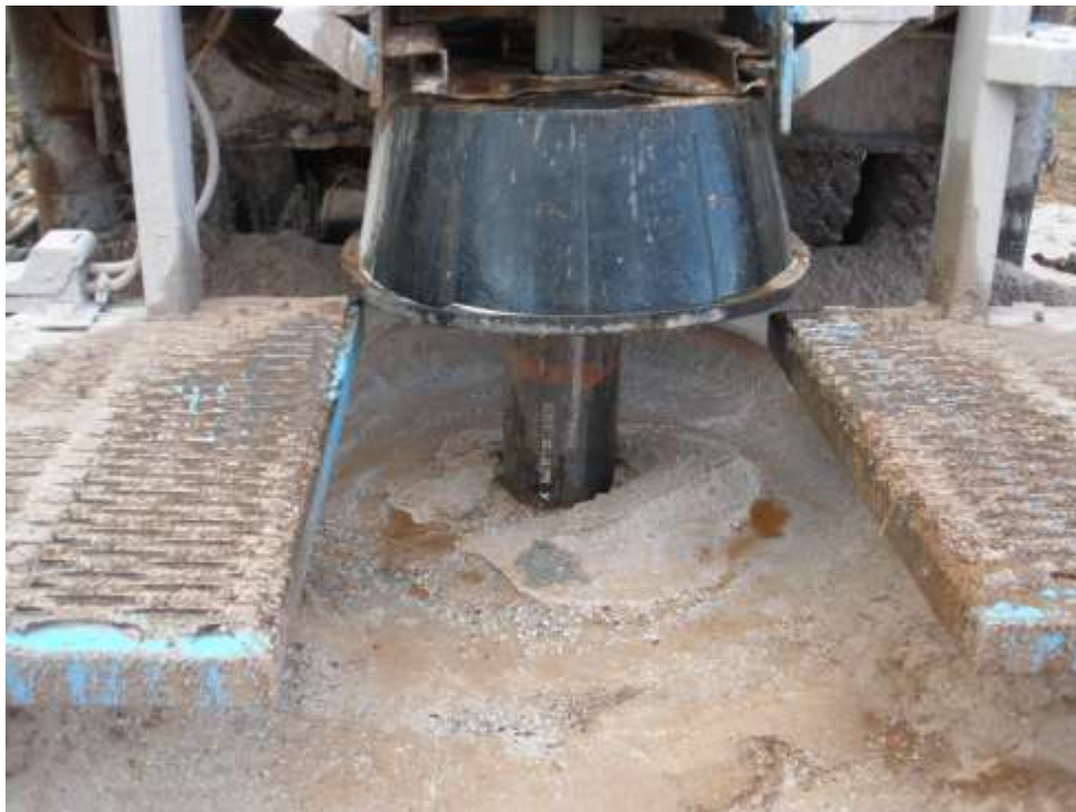
Photo during the airlifting test at the end of drilling. Air was circulating through the drill pipe at 400 \text{ ft}^3/\text{min} . Only a few drips of water are being produced.
