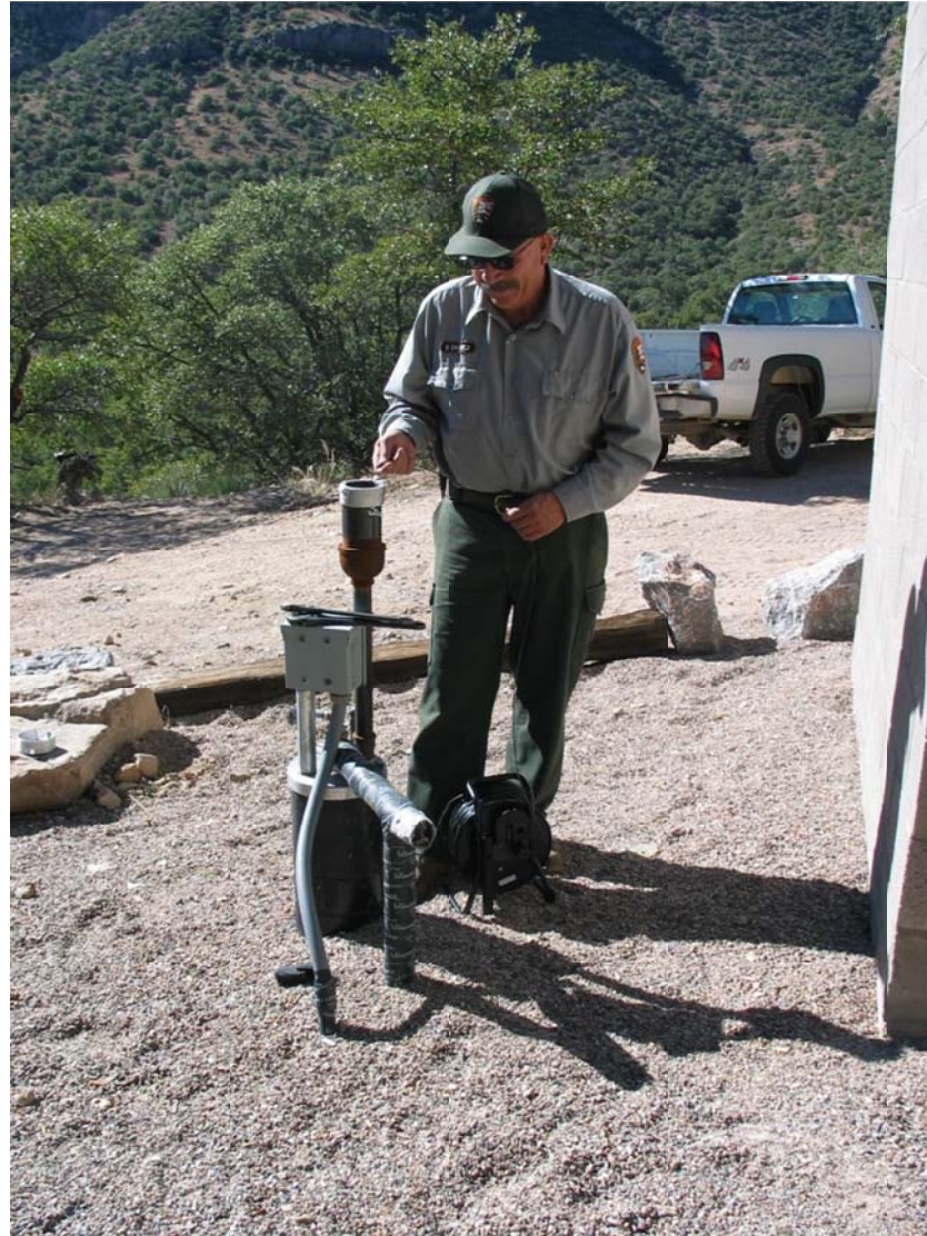
Figure 3. Measuring water level at the CORO-WSW-2 wellhead.
