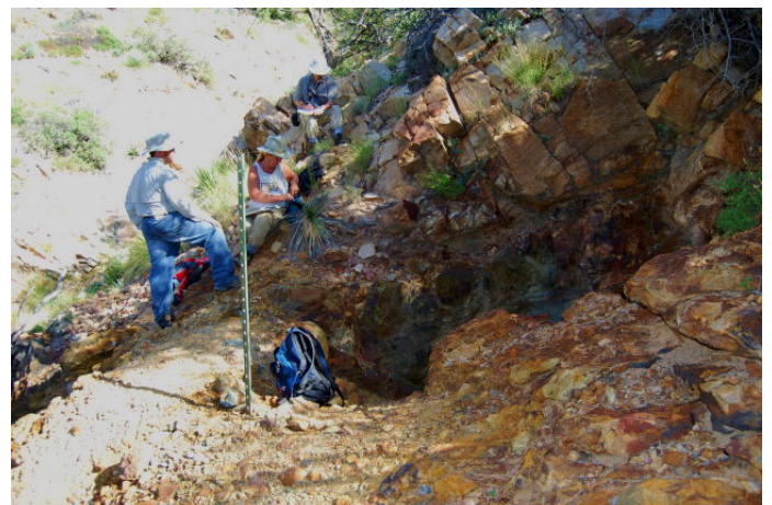
Figure 4. Collar of inclined shaft. High sulfide ore in foreground on mine dump.
