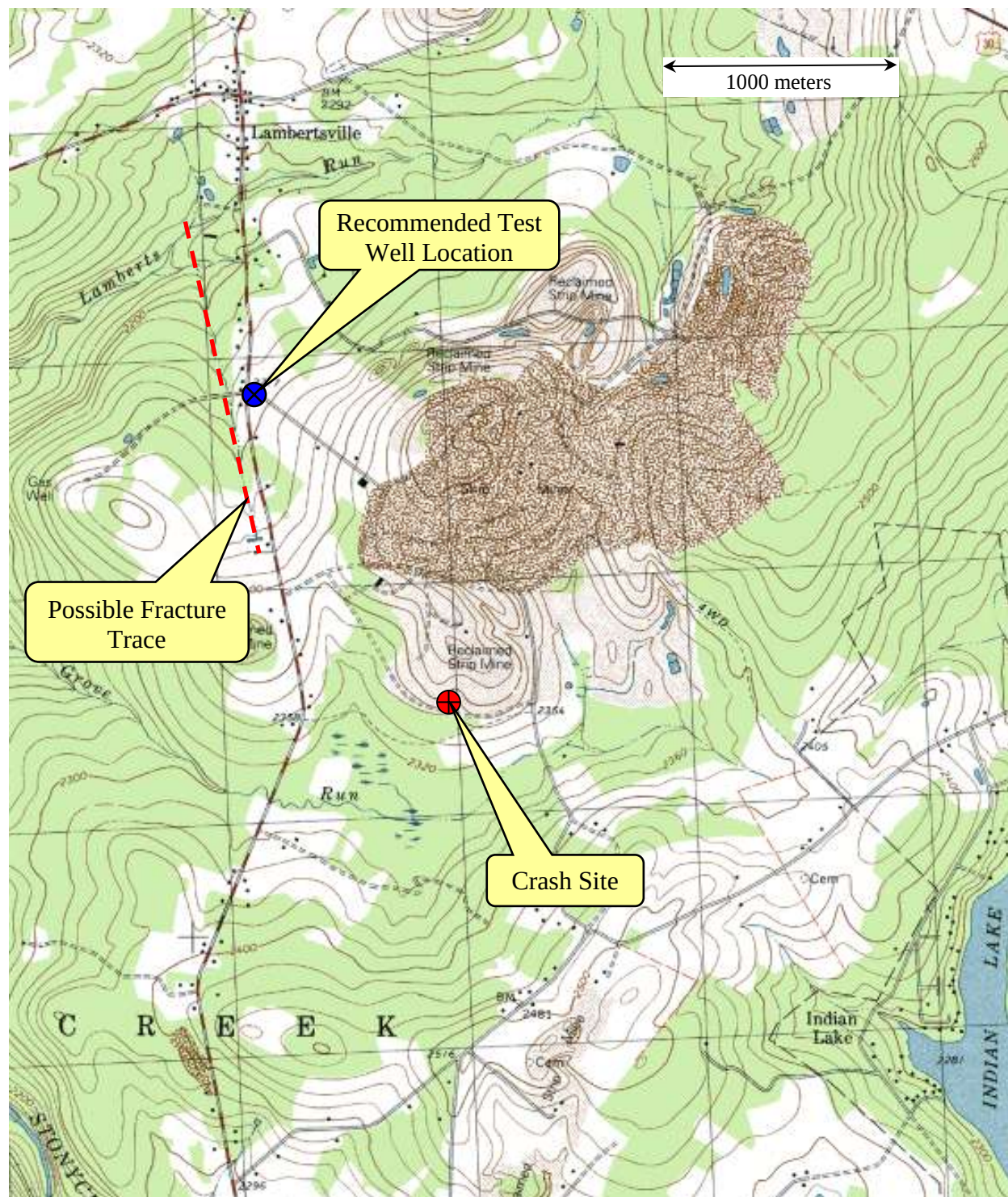
Figure 2. Recommended location of a test well at the Flight 93 National Memorial.
