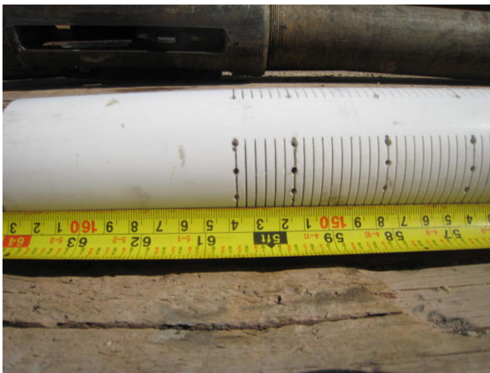
Figure 8. Photograph of the nominal 2-in. diameter well screen showing 3/16-in. holes drilled to enlarge the screen openings for the deep well in fractured marble and granite at well site 1 east of sewage lagoons, Great Basin National Park, White Pine County, Nevada.
