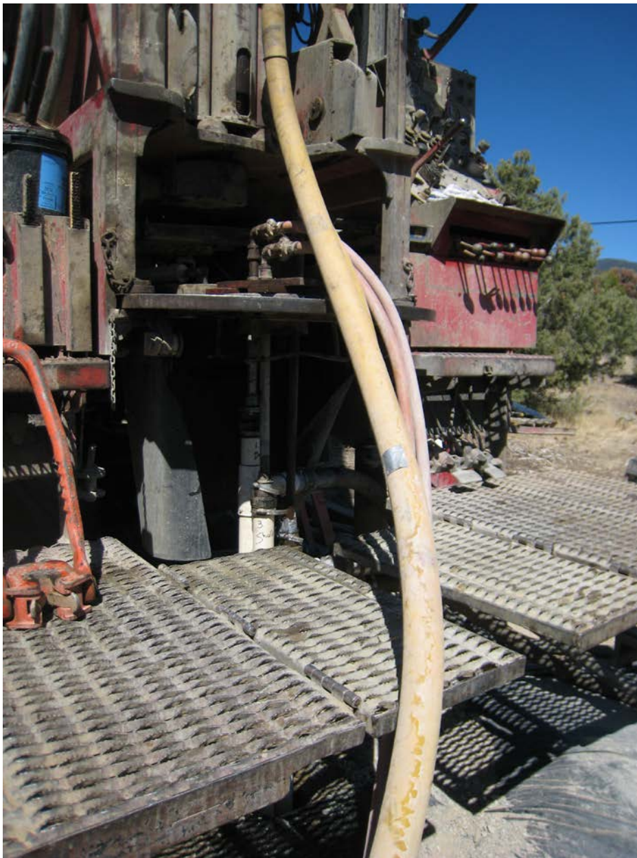
Figure 9. Photograph of the air tubes protruding from each of the three wells used for well development at well site 1 east of sewage lagoons, Great Basin National Park, White Pine County, Nevada.
