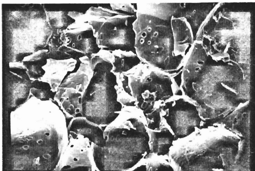
Fig. 35. Longleaf pine twig. Black charred and coated with gold in regular procedure.
