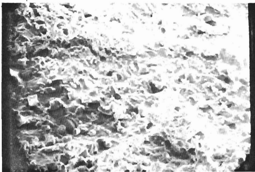
Fig. 94. Bamboo airborne particulate showing both fibrous and cottony structure. 550X.
