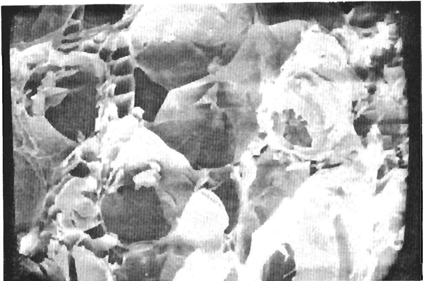
Fig. 27. Edge view of longleaf pine bark scale from regularly control burned forest. Black char. 220X.
