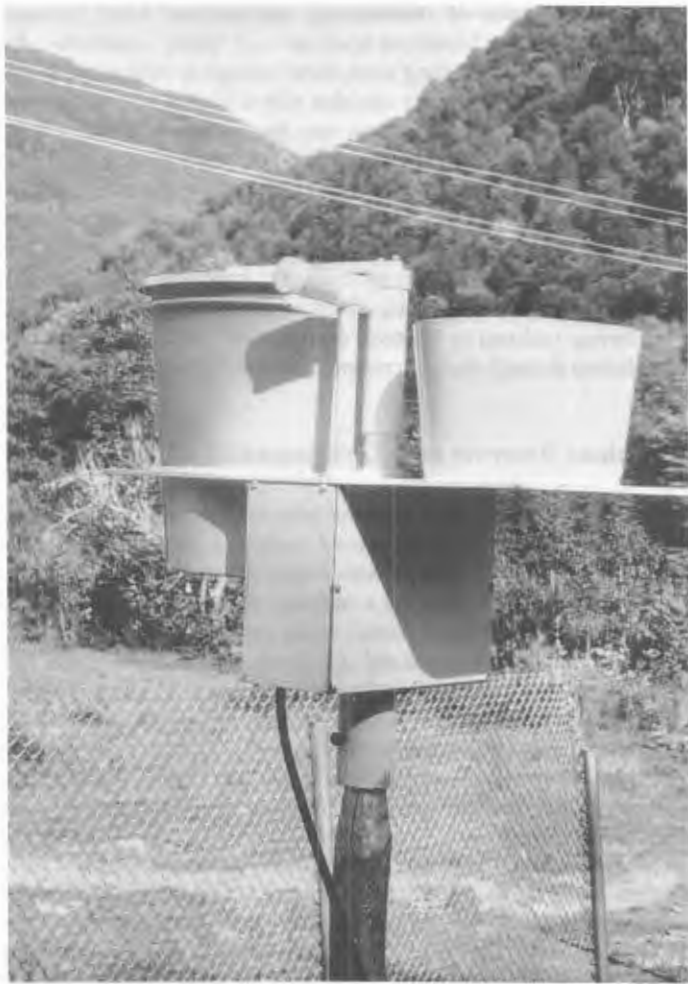
Many biosphere reserves are ideal sites for monitoring baseline changes in airborne pollutants, using sophisticated instrumentation such as this atmospheric sampling device in the Soviet Union's Caucasus Reserve. Photo: C. Wiersma.
