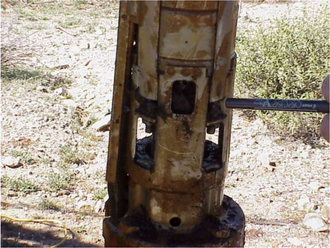
MVC-009L shows plugged intake.
