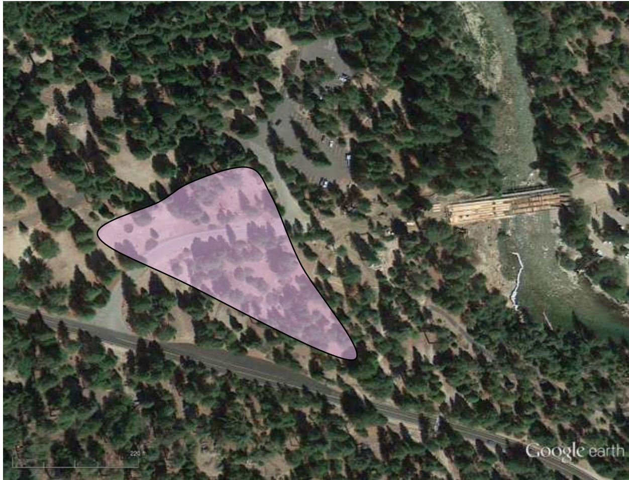
Figure 5. Recommended location for a test well in the alluvial aquifer near Cedar Grove.
