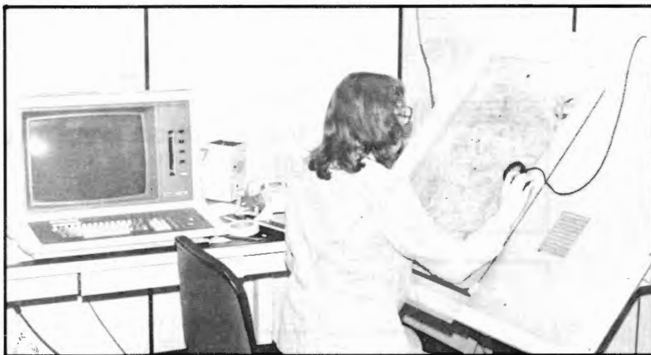
DIGITIZER tablet and graphics display terminal (by which data is digitized to form a digital data base for various kinds of analysis.)
