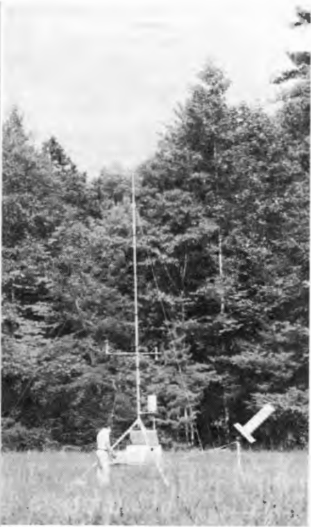
View of the Elkmont CDCP note the tube-shaped GOES antenna to the right of the platform. Weather information (wind speed and direction, relative humidity, rainfall, etc.) is collected by the CDCP and transmitted to the GOES satellite on a 24-hour basis.
