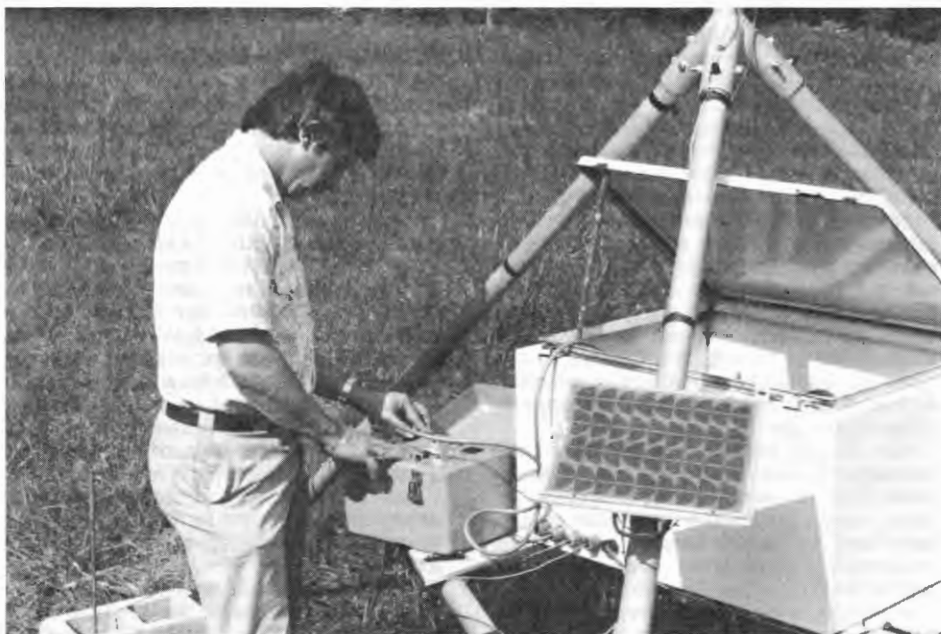
Ray Mathews checks out weather instrumentation on Convertible Data Collection Platform (CDCP) mounted at Elkmont, a low elevation sampling site in GRSM. The CDCP is powered by lead-acid batteries augmented with a recharging system provided by a solar panel.
