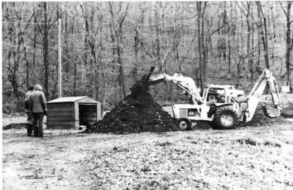
A complete view of the Piedmont District composting site at C & O Canal. Left to right are: shed housing the blower, a compost pile being constructed, a blanket of compost being added to the wet mixture to insulate against excessive heat loss, protect from rainfall and reduce odor. Behind the tractor is a working static compost pile. The storage tank with concrete mixing apron in front of it is at the extreme right. The slope around the site diverts runoff to a holding basin in the photo foreground.
