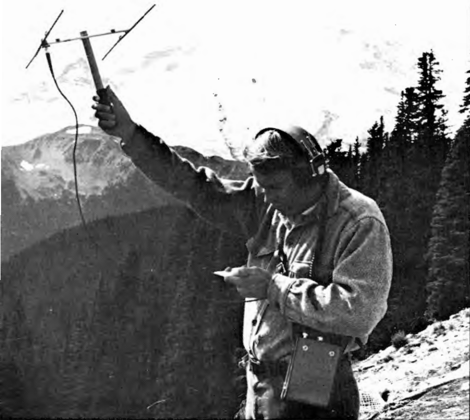
Holding the antenna and wearing a techtronics radio locator, Alan Ewert monitors a radio-collared elk.
