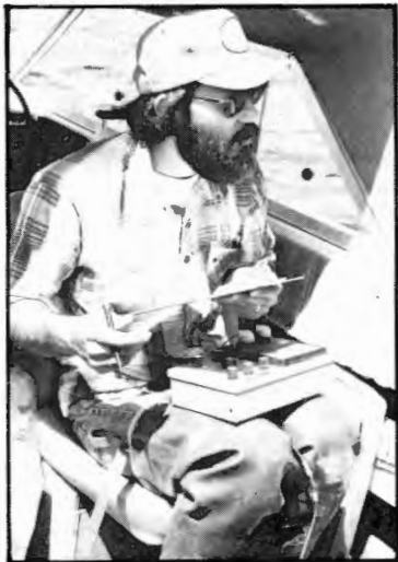
Steve Sumioka, USGS, balances his combination temperature and dissolved oxygen probe and records information from the surface to the 132-foot deep bottom of Spirit Lake.
