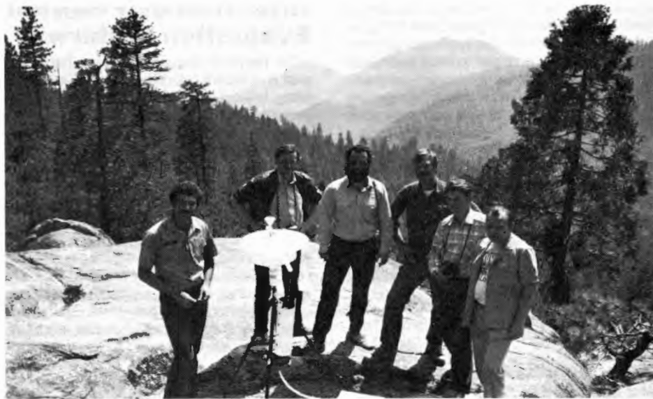
On a Sierran bald at about the 7000-foot level, an atmospheric group inspects the precipitation event collector for chemical analyses. From left, Dan Drisco, Sequoia/Kings Canyon NP resource management specialist; Kirill D. Zykov, Ray Herrmann, NPS Water Resources Lab Chief; Yuri A. Starikov, Valery A. Petrukhin, and Yuri G. Puzachenko. The Russian participants in the pulse study were there courtesy of the U.S./U.S.S.R. Bilateral Environmental Agreement.
