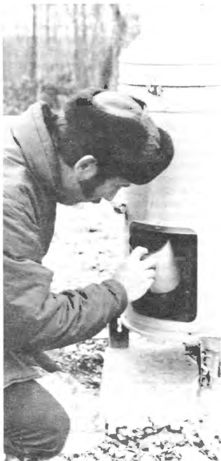
A resource management technician at Buffalo National River replaces the drum graph in the NADP recording rain gauge. The instrument charts the intensity and duration of each rain or snow shower which falls on the sampling site.
