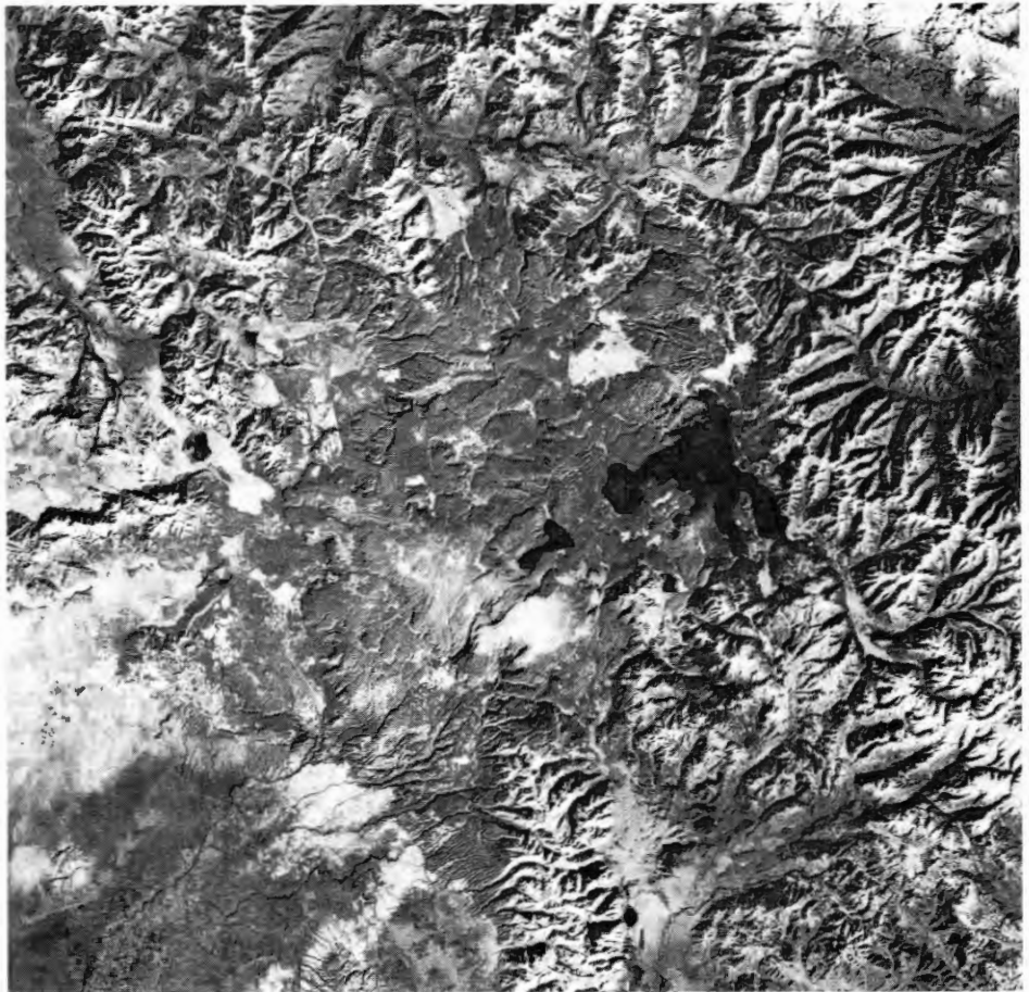
LANDSAT-1 satellite scene shown here covers most of the greater Yellowstone ecosystem. The image was obtained Nov. 23, 1972 in the photographic infrared portion of the electromagnetic spectrum (MSS channel 7). This type of data is used by the NPS as a tool for inventorying and managing park resources via digital image processing and computerized geographic information systems (GIS).
