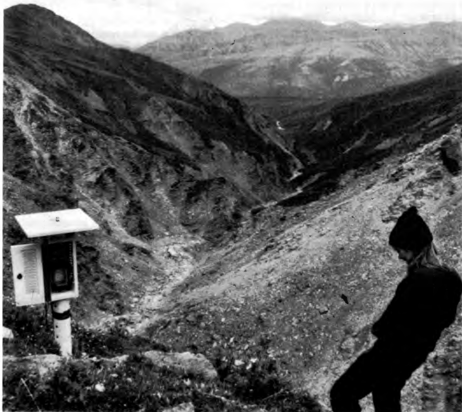
Figure 2. Remote automated monitoring station to assess effect of temperature, moisture, and radiation on vegetation production, decomposition, and nutrient cycling.
