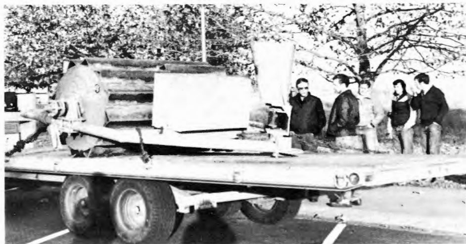
Power seeder by John Deere, designed to drill and plant seeds at least 1/4 to one inch underground, is shown here mounted on a flatbed truck. The power seeder, pulled by a tractor, is capable of precise placement of seeds — where you want them and out of the sight of feeding birds.
