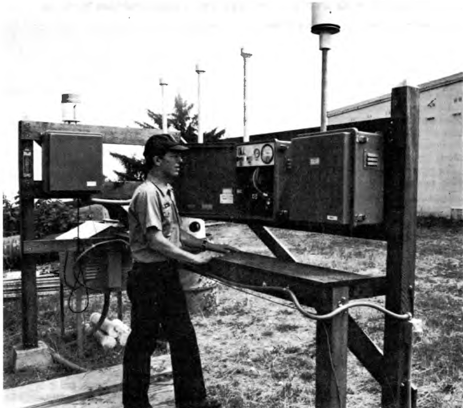
John Sacklin, at Redwood NP, is shown with the IMPROVE (Interagency Monitoring of PROtected Visual Environments) particulate sampler. The IMPROVE program is designed to determine extent and causes of visibility impairment at selected Class I clean air areas throughout the United States. The cooperative program involves several federal agencies including the NPS. The monitor automatically takes 24-hour samples on Wednesdays and Saturdays. These are analyzed for trace elements, mass, ions, and carbon.
