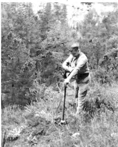
Figure 1. Reading the natural potential on a slope of Hell Canyon directly outside the natural portal of Jewel Cave.
