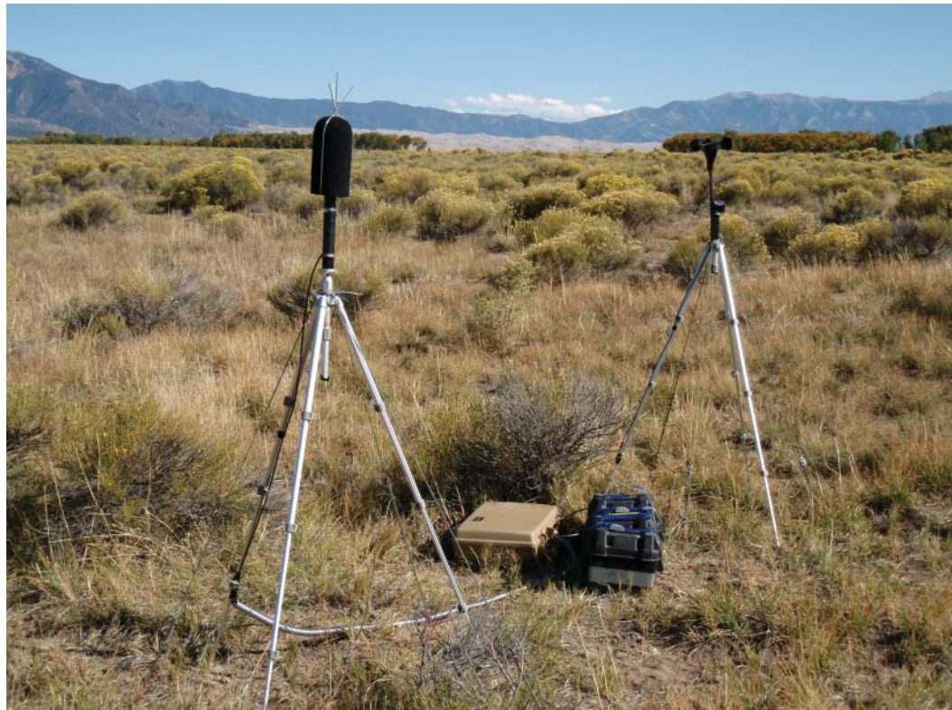
Figure 3. Acoustic monitoring station deployed at Great Sand Dunes National Park and Preserve, Colorado. The anemometer on the right is used to determine when wind speeds are too high to obtain reliable measurements. The microphone on the left is topped with a metal spike to discourage birds from perching on the foam windscreens. The unit costs about $10,000. Data collected at this site were used to document extraordinarily quiet conditions in the park, which were important in subsequent discussions regarding oil and gas development near the park (NPS/Emma Lynch).
